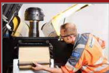
Gull wing hoods provide quick access
