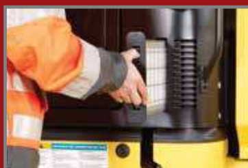
Interior cabin filter ease of access
