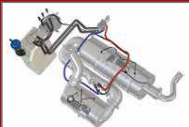
Tier 4 Final after-treatment package
