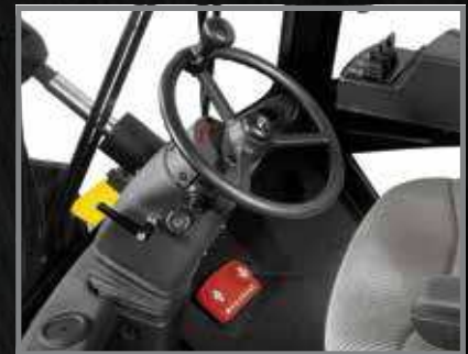
Fully adjustable steering column
