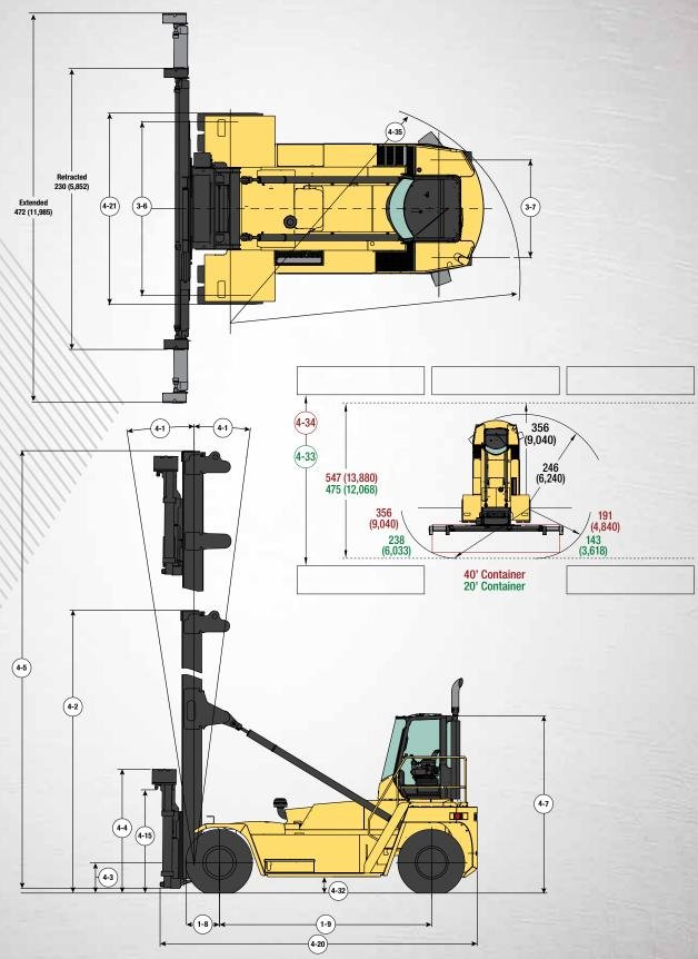
Circled dimensions correspond to the line numbers on the tabulated chart inside the Technical Guide. Dimensions are in inches (millimeters).
