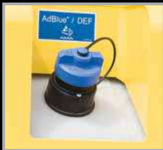
Diesel Exhaust Fluid (DEF) tank.
