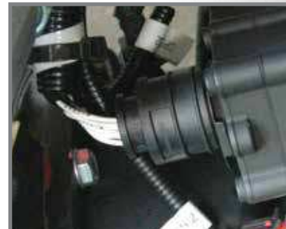
Standard profile Deutsch pin connectors, IP64 compliant
