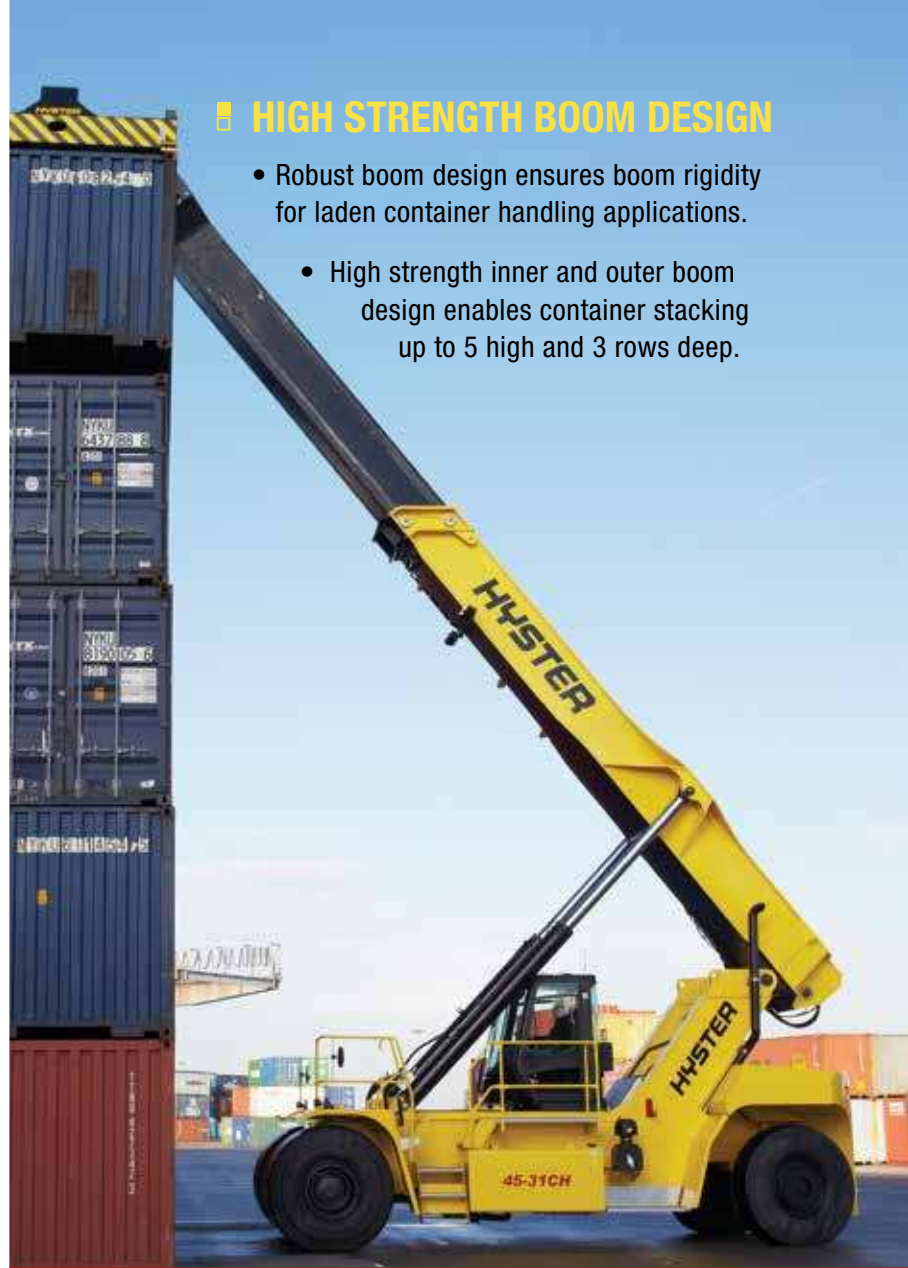
Durable 2-stage boom design constructed with T-1 steel, with two plane welding for added boom strength
