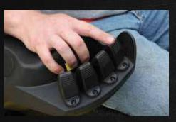
Adjustable armrest that accompanies the optional TouchPoint e-hydraulic control moves with the seat and telescopes forward/vertical in one simple movement to provide greater flexibility in achieving a more custom position.
