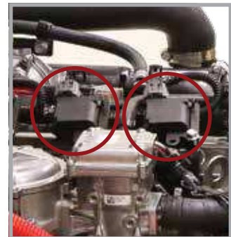
Coil over plug ignition design
