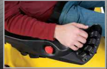
Electro-Hydraulic Controls with Touchpoint Mini-Levers
