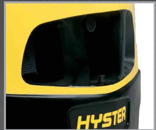
Counterweight tunnel design improves airflow
