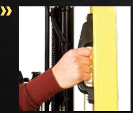
An optional rear drive handle with horn button makes reverse operation easier.
