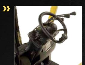
The 12-inch steering wheel rests on a tilting steer column, offering infinite adjustments and comfort.
