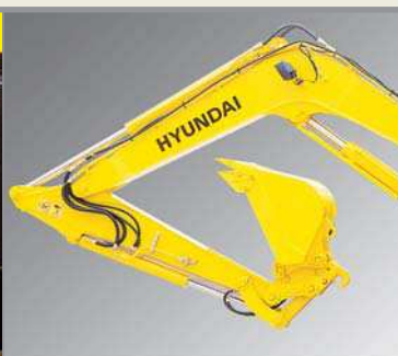
Installation for Breaker Operation
