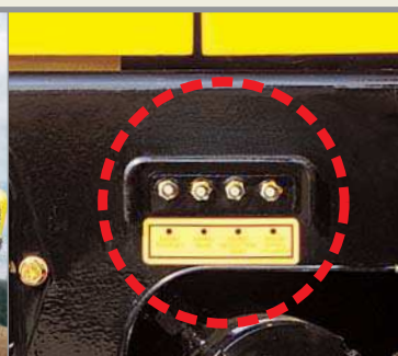
Centralized Grease Fittings
