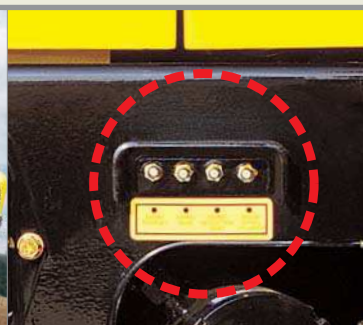
Centralized Grease Fittings
