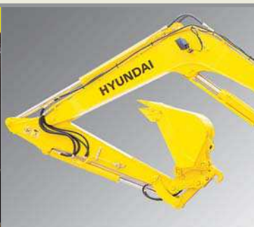
Installation for Breaker Operation
