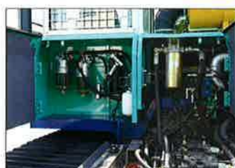
Fuel pump, Fuel filter, Hydraulic filter
