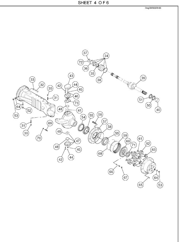
AXLE 4-WHEEL DRIVE STEERING (59251652) - INTERNAL BREAKDOWN SHEET 4 O F 6
