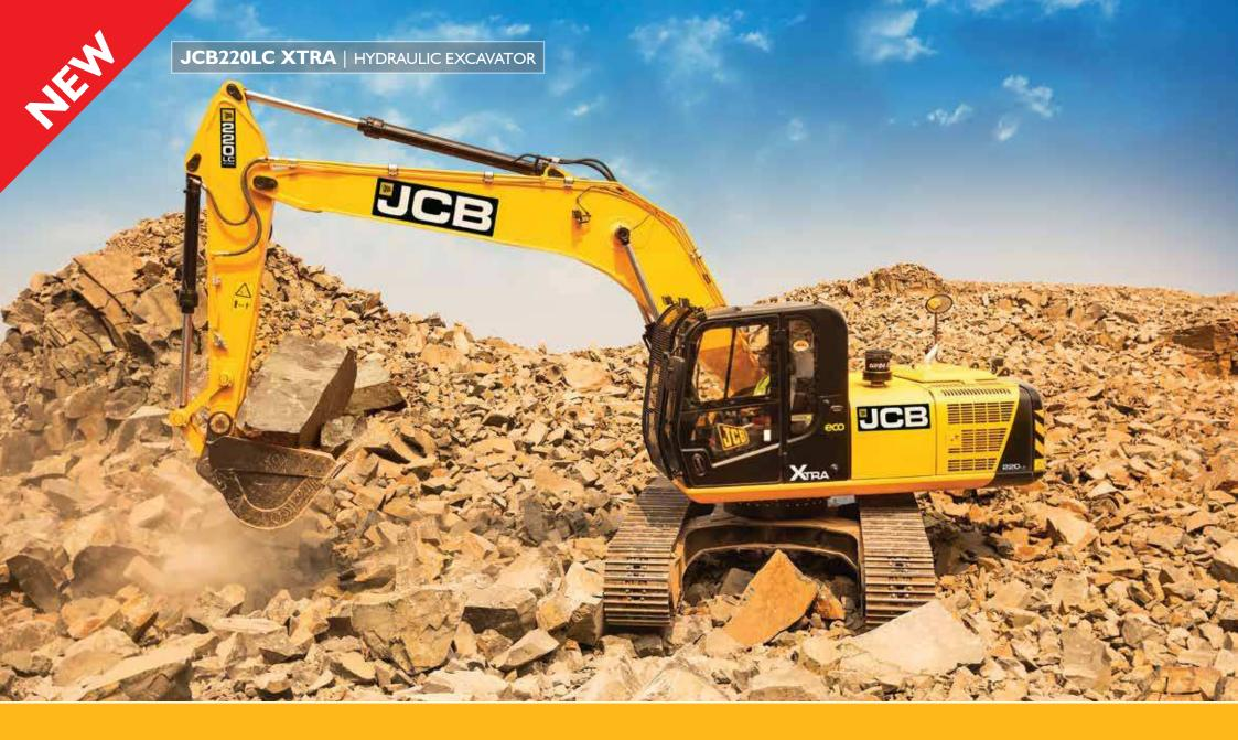
Engine Power : 170 hp (127 kW) Bucket Capacity : 0.8 cu.m - 1.2 cu.m Operating Weight : 21750 Kg
