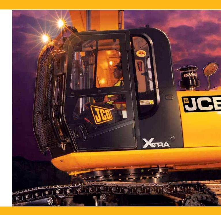
The deluxe operator seat provides a high level of seating comfort. While the seat is adjustable for weight, seating angle, forward and backward movement and back rest angle it can be moved along with the joystick to ensure best position of operator with respect to the controls for fatigue free operation.
