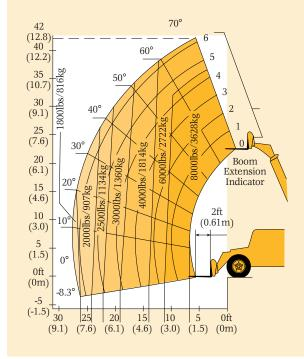
Lifting performance and stability conform to ANSI B56.6 1992. The load chart capacities relate to a standard machine equipped with standard 48in. (1.22m) pallet forks. The use of any attachment **reduces** the load capacity of the machine. Always refer to the **load charts** placed in the machine prior to lifting or placing
