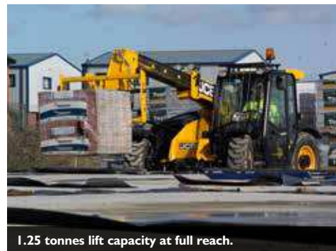
Fast and precise control with single lever servo control and proportional auxiliaries.
