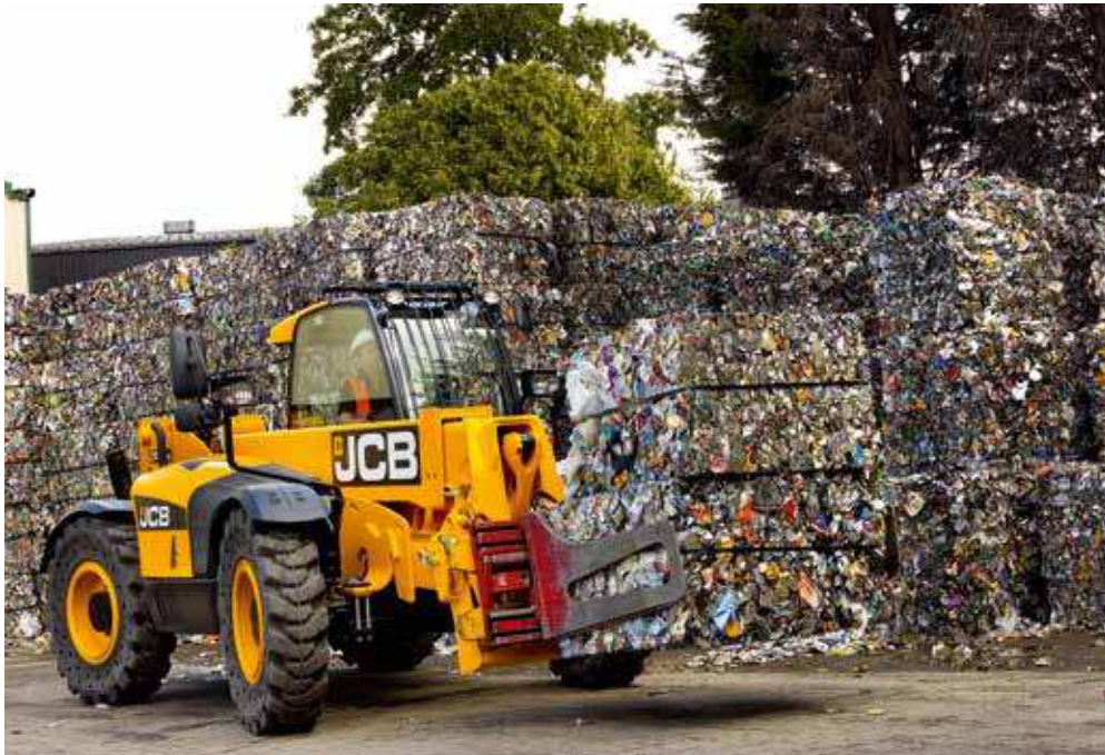
Best-in-class comfort with one of the largest cabs in the industry. The cab conforms to ROPS ISO 3471 and FOPS ISO 3449 and puts the operator firmly in control.
