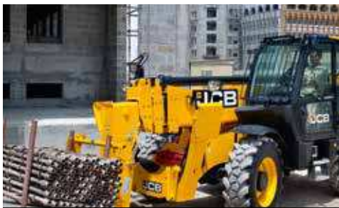
JCB quickhitch system makes changing attachments quick and easy.
