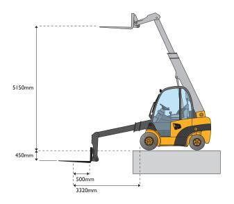
Ordinary lift trucks use hydraulic power for the lift cycle only, and then gravity to lower. But the JCB Teletruk uses full hydraulic power down too; and this can be put to good use for specialist applications such as loading ships stores.
