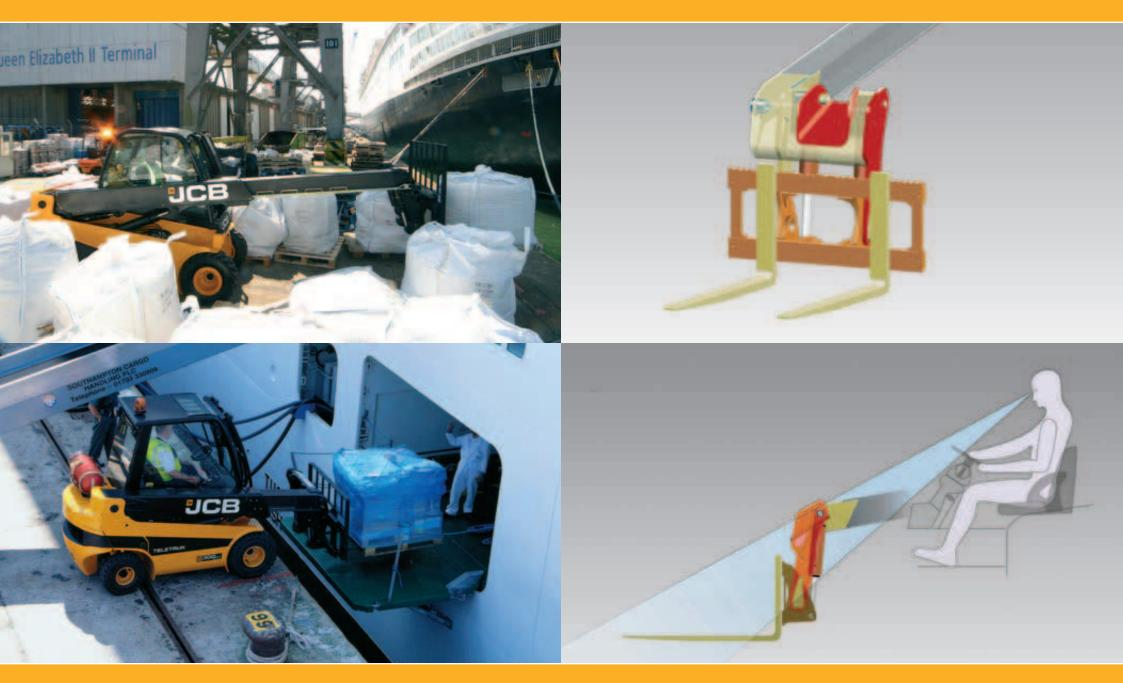
The JCB Teletruk range comprises ten compact models with diesel powered fully-enclosed hydrostatic drivelines in two and four-wheel-drive, and two Gas (LPG) powered two-wheel-drive models.
