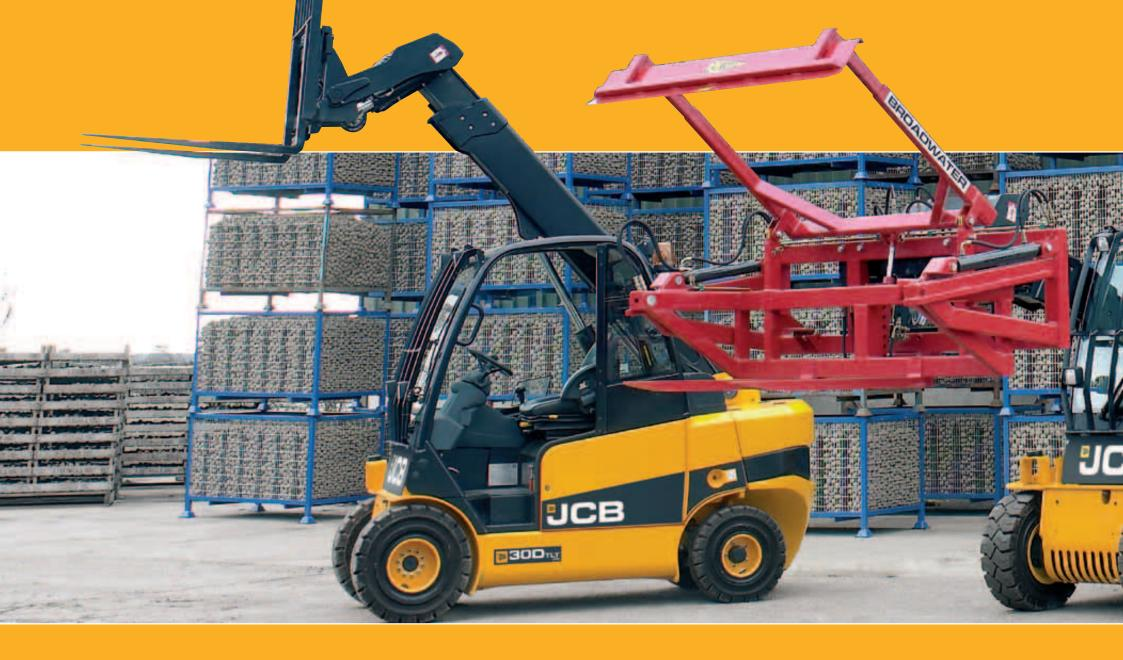
First take the small footprint of an industrial counterbalanced lift truck. Then add the telescopic boom of a telescopic handler. Design-in a fully enclosed hydrostatic drive system. Then finish off with a hydraulic quick-disconnect carriage for forks or shovel. Well that's what we've done at JCB to bring you the JCB Teletruk Range; the world's
