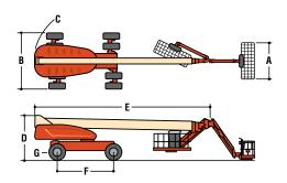
**Standard Features** Platform: 36 x 96 in. (0.91 x 2.44 m) Side Entry 8 ft (2.44 m) JibPLUS® Boom Selectable Capacity Envelope 180° Hydraulic Platform Rotator AC Receptacle in the Platform 5 Degree Tilt Alarm/Indicator Light All Motion Alarm Swing-Out Engine Tray 12V DC Auxiliary Power Hourmeter Control ADE° System Full-time 4WD 3 Selectable Steering Modes
