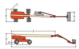
**Standard Features** Platform: 36 x 96 in. (0.91 x 2.44 m) Side Entry 8 ft (2.44 m) JibPLUS° Boom Selectable Capacity Envelope 180° Hydraulic Platform Rotator AC Receptacle in the Platform 5 Degree Tilt Alarm/Indicator Light All Motion Alarm Swing-Out Engine Tray 12V DC Auxiliary Power Hourmeter Control ADE® System Full-time 4WD 3 Selectable Steering Modes Drive-out Extendible Axles Oscillating Axle **Proportional Controls Gull-Wing Hoods** 445/50D710 Foam Filled Rim Protector Lug Tread Tires
