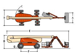
**Standard Features** Platform: 36 x 96 in. (0.91 x 2.44 m) Side Entry 8 ft (2.44 m) JibPLUS® Boom Selectable Capacity Envelope 180° Hydraulic Platform Rotator AC Receptacle in the Platform 5 Degree Tilt Alarm/Indicator Light All Motion Alarm Swing-Out Engine Tray 12V DC Auxiliary Power Hourmeter Control ADE® System Full-time 4WD 3 Selectable Steering Modes Drive-out Extendible Axles Oscillating Axle
