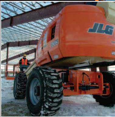
Oscillating Axle For Improved Traction & Drive Performance
