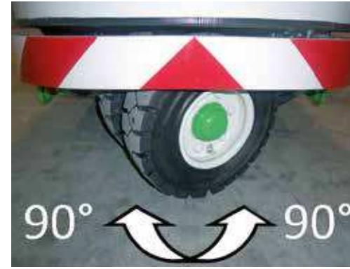
REAR 90°+90° AND COUNTER ROTATION SYSTEM ON FRONT WHEELS
