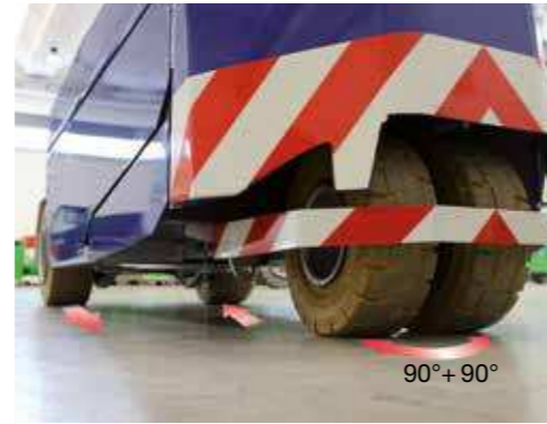
STEERING 90°+90° AND COUNTER ROTATION SYSTEM ON FRONT WHEELS
