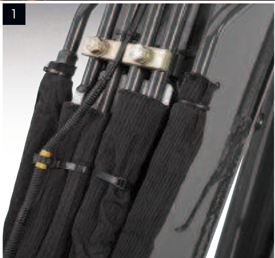
1. Steel hydraulic lines are clamped securely; Cordura® covering on rubber hoses provides extra durability.
