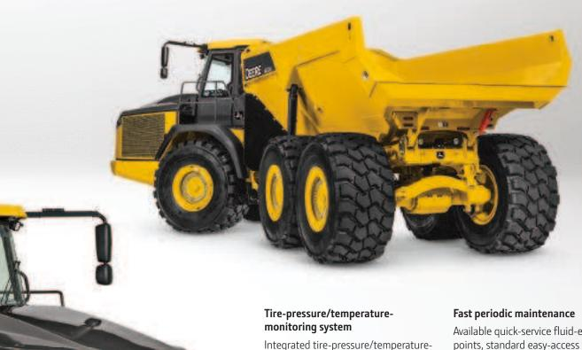
Integrated tire-pressure/temperature-monitoring system comes standard to help maximize tire life and fuel efficiency. If pressure drops by 10 percent, a passive alarm appears on the monitor. Further decreases or overheating result in an audible warning, and an email alert is sent to you via JDLink.
