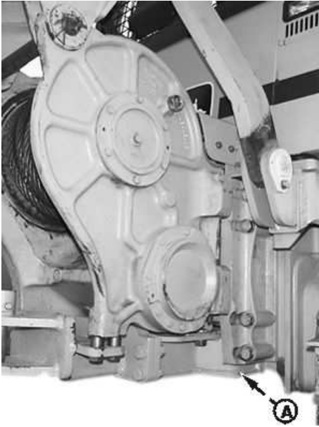
Winch Oil Filter Location
