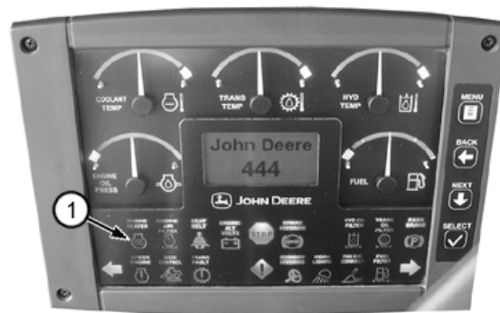
1—Engine Heater Indicator
