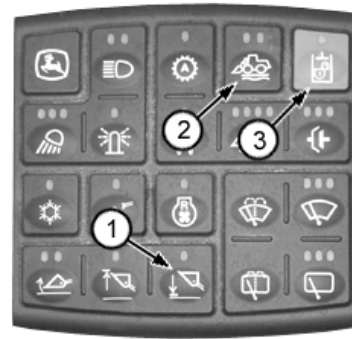
1— Return-to-Carry Switch 2— Ride Control Switch
