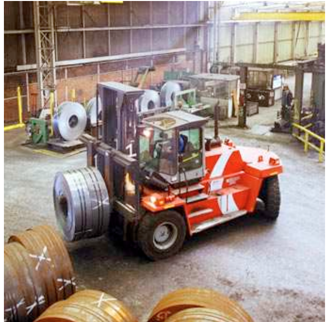
DCD240-6LB with coil ram in steel operation.
