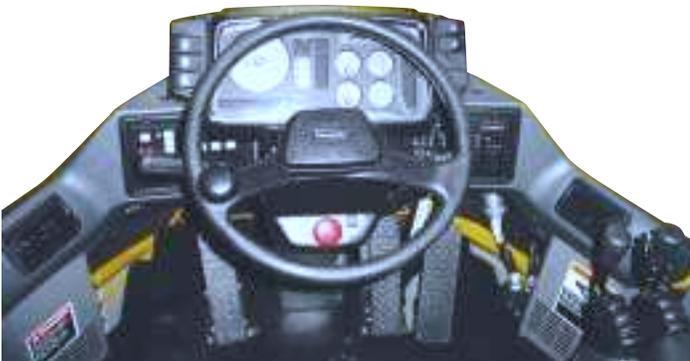
***Easy-to-read gauges and adjustable telescopic and tilt-steering with attached instrument panel provide accurate information at a glance.***
