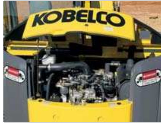
The engine hood easily swings open to provide complete access for routine maintenance.
