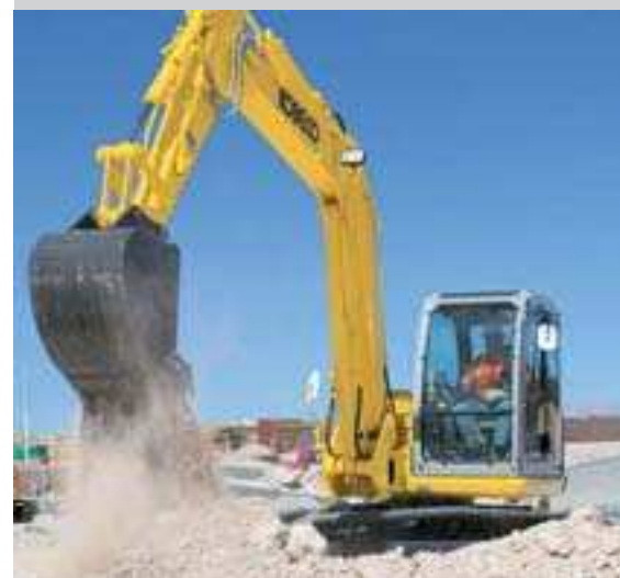
The Kobelco swing system uses a swing shockless valve that absorbs and dampens the effect of each rebound. You get smoother starts and stops, and more precise bucket placement.
