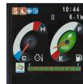
DEF tank level gauge
