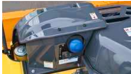
Urea tank Urea filler cap is placed on the step for easy access.
