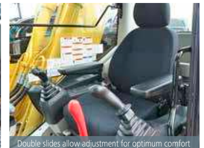
Double slides allow adjustment for optimum comfort
