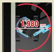
The SK17SR features a larger swing angle of 65 degrees left and 55 degrees right.
