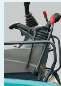
Safety lever lock permits enter and exit only when the levers are disengaged to prevent accidental operation.
