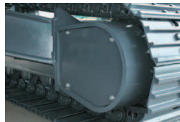
Reinforced travel motor cover A reinforced travel motor cover is used to protect critical hydraulic motor components.
