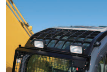
Top guard level II (Meets ISO10262) The standard feature of the grid type cab ceiling guard protects the operator against objects falling on the cab roof.
