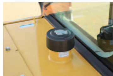
Dust-proof fuel tank cap The fuel cap is lined with rubber so that dust does not easily contaminate the fuel tank.
