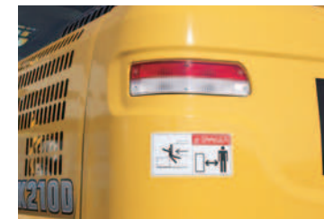
Rear swing flashers and rear work lights The swing warning lamp helps prevent collisions and accidents where workers are trapped while the upper body is turning.
