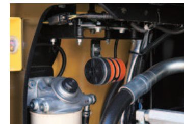
Travel alarm When traveling onsite, the standard alarm function cautions workers in the area with an electronic sound.
