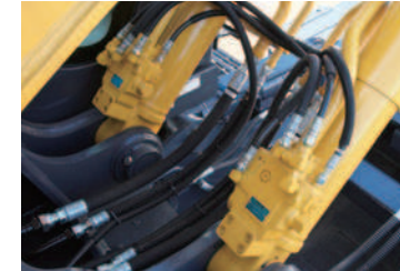
Boom holding valve The standard boom fall prevention valve provides protection against unexpected breaks in the boom cylinder piping.
