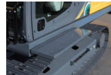
Catwalk The larger step makes it easy for the operator to climb into and out of the cab.
