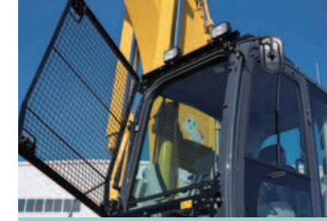
Glazing with shatterproof film The windshield and right window are provided with shatterproof film that prevents loose glass chips from scattering even if it is smashed.
