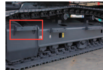
Lower frame step An additional step is installed on the side of the crawler frame.
