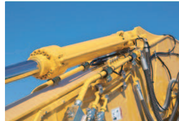
Dismantling bucket cylinder Use of a dedicated cylinder with reinforced components.
