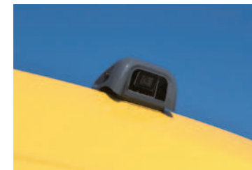
Rear view camera The view from behind the machine can be displayed with camera images on the multi-display.
