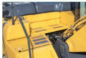
Maintenance space The upper space provides a comfortable platform for maintenance inside the engine hood.
