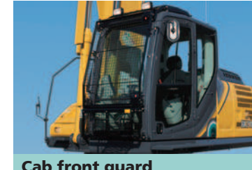
Cab front guard The windshield and the lower window are provided with a vertical grid guard of radial design so as not to block the operator's field of view. The quick open/close design makes cleaning easy.
