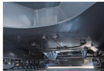
Lower undercover The lower car body structure is fitted underneath with a 3/8" (9 mm) thick reinforced cover.
