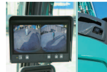
Additional right camera + monitor The view from the right side of the machine can be confirmed on the standalone monitor to exclude blind spots. Optional
