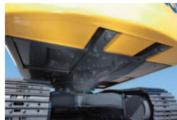
Upper main body undercover The 1/4" (6 mm) undercover guards protect critical hydraulic and electrical components.
