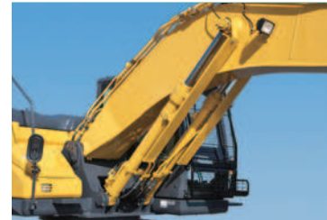
Boom cylinder guard Protects boom cylinder rods.
