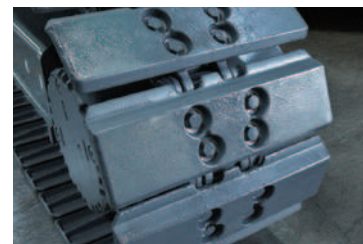
Flat shoes Flat shoes that are durable against wear on concrete sites are selectable as the option. Optional
