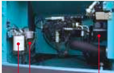
Additional large water separator Large fuel filter (with built-in water separator)
