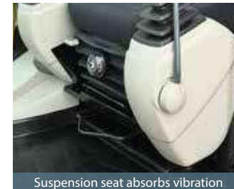
Suspension seat absorbs vibration
