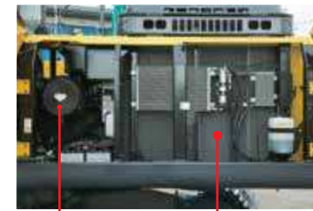
Air Cleaner (double element) Radiator
