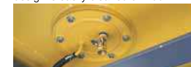
Fuel tank drain valve.
