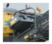
• MUCK CONVEYOR: Muck conveyor assembly can be folded by hydraulic cylinder, 3414 mm x 600 mm 11'2" x 2'
