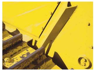
Chassis Deflector Bars and Bolt Guards Help protect and keep debris away from components.
