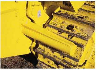
Trapezoidal Track Shoe Holes Minimize debris packing and extend track component life.
