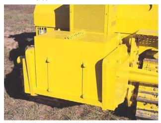
Landfill Counterweight Optimizes machine balance for landfill applications.
