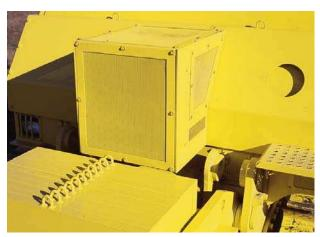
**Rear Mounted Hydraulic Cooler and Fan** Relocated from the engine compartment to increase cooling efficiency.
