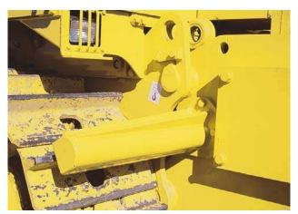
Front and Rear Striker Bars Help prevent debris from riding up onto the track and damaging the fenders or chassis. Bolt-on for easy maintenance.
