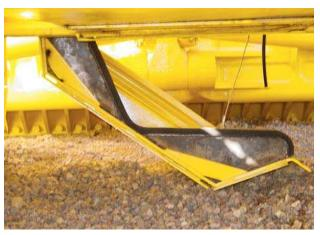
**Engine Bottom Guard With Electric Winch** Simplifies cleaning of the engine compartment.
