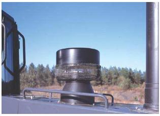
**Turbine Pre-Cleaner** Helps remove particulates from the engine air before they reach the filter elements.
