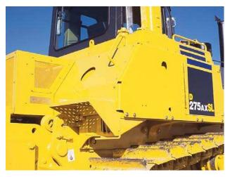
**Fuel and Hydraulic Tank Guard** Helps protect these components from damage and debris. Hinged covers allow access for cleaning and maintenance.
