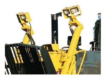
Supplemental Lighting Guarded lights are raised to optimize lighting for machines equipped with a trash blade.
