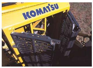
Hinged Radiator Door Quick opening two-piece doors allow easy access to the radiator and fan for cleaning.
