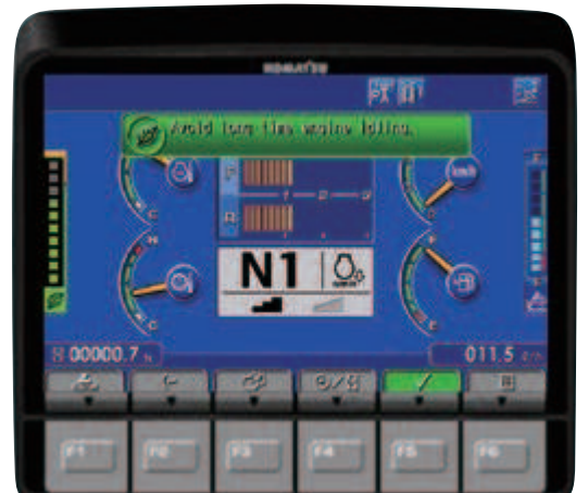
Eco gauge, eco guidance and the new auto idle stop help to further reduce consumption.
