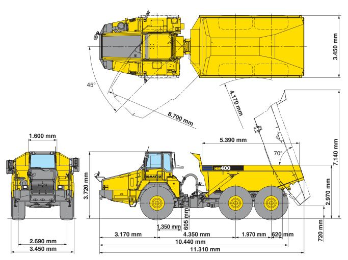
All measurements with tyres 29.5 R25; if equipped with tyres 875/65 R29: Overall height 3.740 mm, overall width 3.665 mm, tread 2.805 mm
