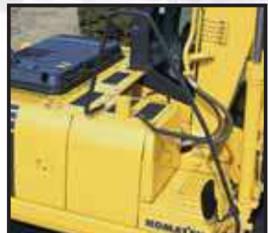
Large handrail for safe access
