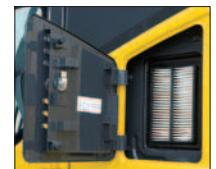
External air conditioner filter
