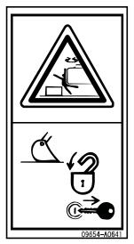
Sign indicates a hazard of being caused or run over by unexpected moving of stopped machine.
