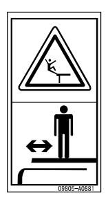
Sign indicates a hazard of falling off the fender or hood.
