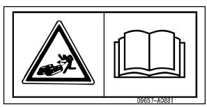
Sign indicates a hazard of flying plug from track adjuster that could cause injury.
