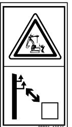
Sign indicates an electrocution hazard if machine is brought too near electric power lines.
