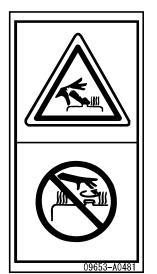
Sign indicates a burn hazard from spurting hot water or oil if radiator or hydraulic tank is uncapped while hot.
