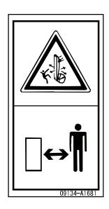
Sign indicates a hazard of being hit by the working device of the machine.
