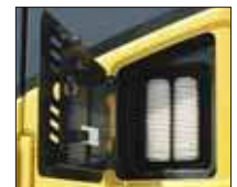
External air conditioner filter
