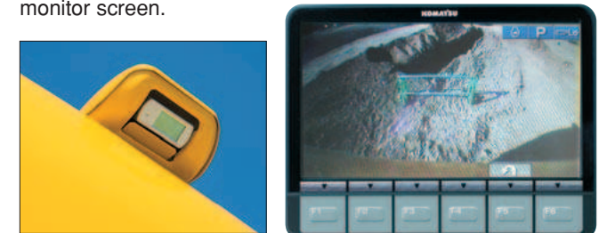
Monitor for rear view camera
