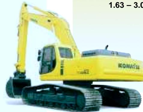
**Comfortable Cab** Komatsu's low-noise cab design uses viscous cab mounts for reduced noise and vibration.
