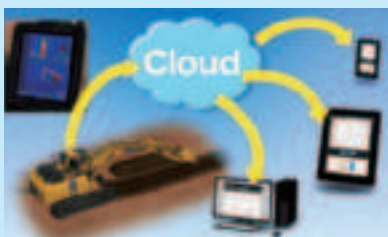
Progress information and as-built data can be sent to the office from the machine in real time.
