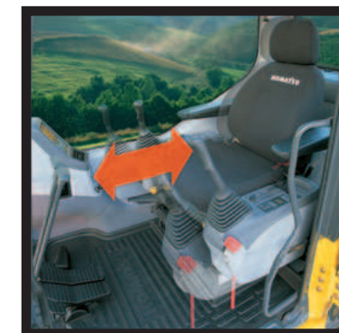
Seat Sliding Amount: 340 mm 13.4", increased 120 mm 4.7"
