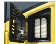
External air conditioner filter
