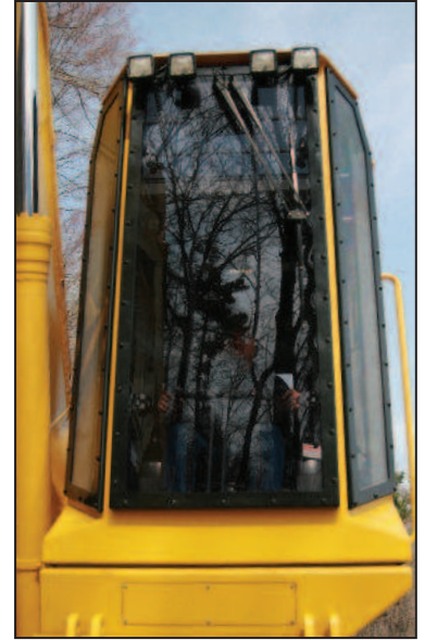
Komatsu purpose-built forestry cab wet arm wiper and 12mm polycarbonate windows. Optional 1 1/4" 32mm window available for processing head applications. (1 1/4" front window shown)
