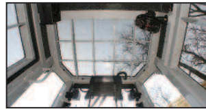
Komatsu purpose-built forestry cab features large color display, climate control, large skylight, 3 12v power points, AM/FM/CD stereo radio and 5 lb fire extinguisher.
