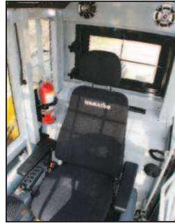
Komatsu purpose-built forestry cab features large color display, climate control, large skylight, 3 12v power points, AM/FM/CD stereo radio and 5 lb fire extinguisher.
