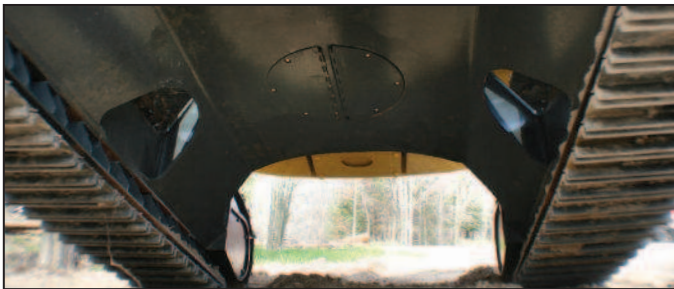
Special high/wide carbod body with PC300 class final drives and undercarriage components provide high gradeability and tractive effort. Heavy duty engine and hydraulic pump compartment service access doors, full length walkways, right hand log guard.
