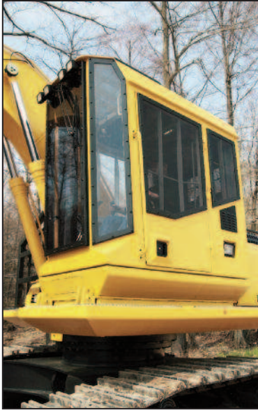
Komatsu purpose-built forestry cab, OPS/TOPS compliant with 8" cab riser cab riser.
