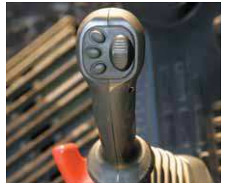
Joysticks with proportional control button for attachments
